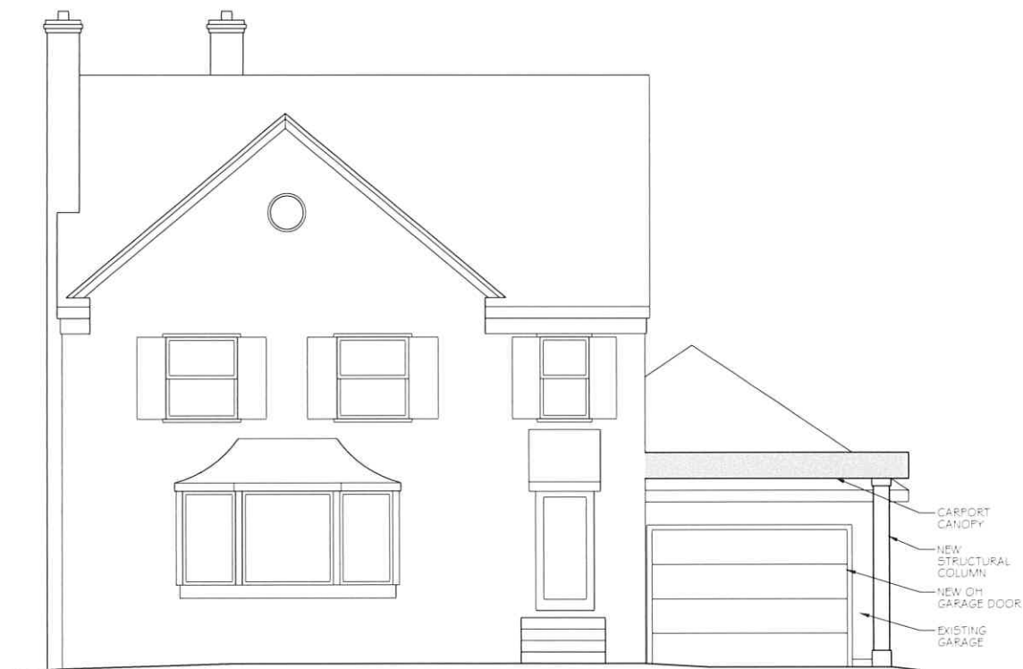
PROPOSED EAST (front) ELEVATION SCALE: 1/4" = 1'-0"
