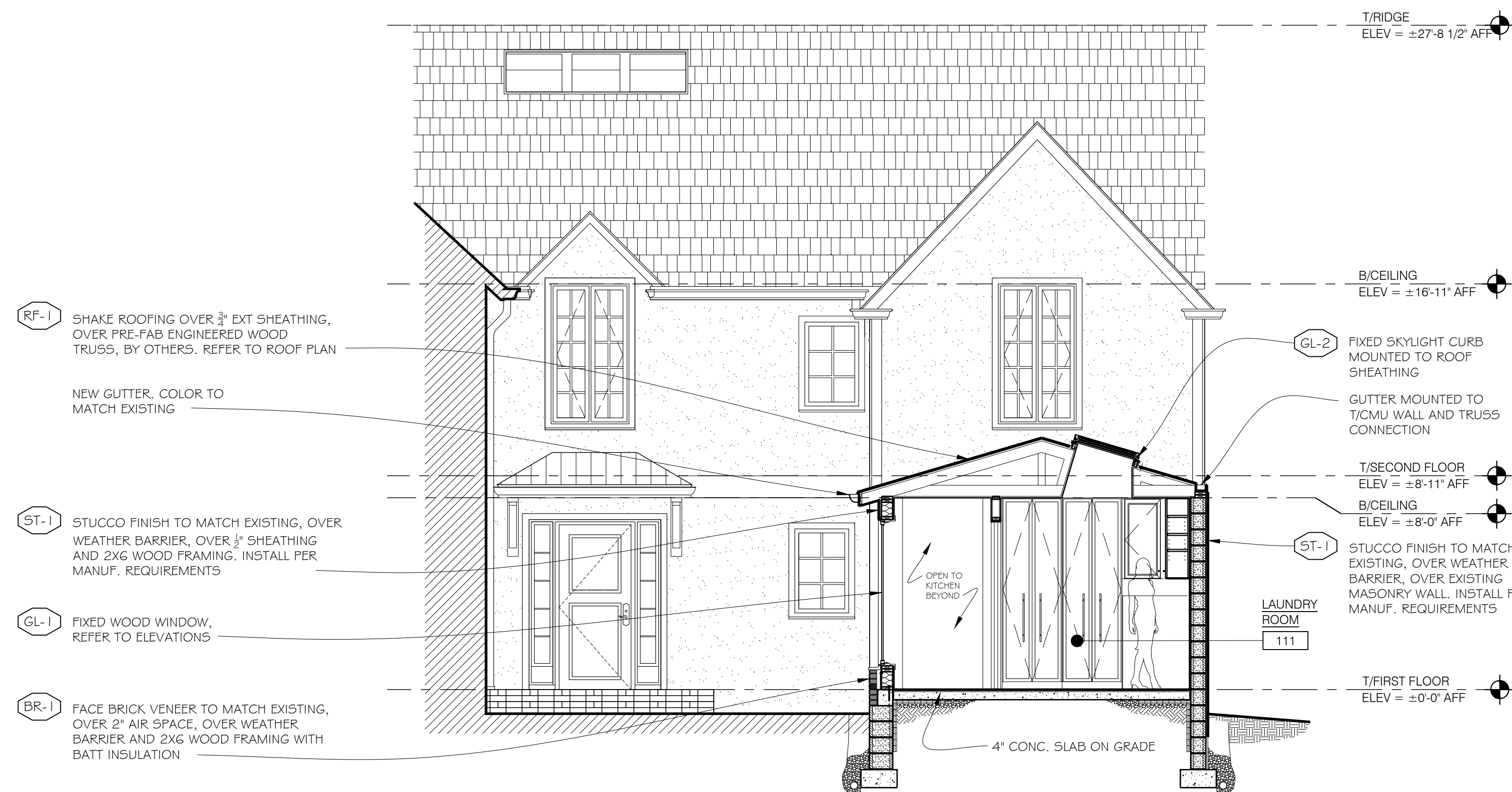
1 A3-01 SECTION FIRST FLOOR ADDITION SCALE: 1/4" = 1'-0"
