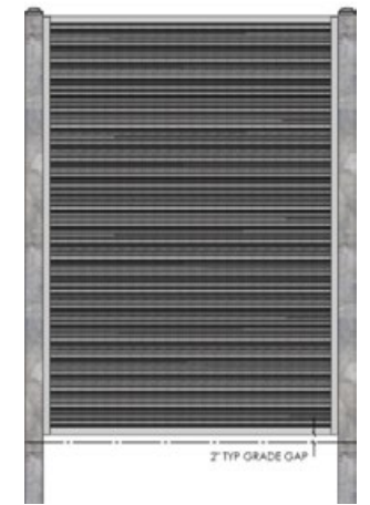
SITE FENCE - METAL 6'-0" H FENCE FINISH
