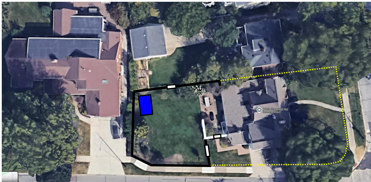
Figure 1. Aerial view of 1100 Elmwood Rd showing existing fence layout. Black = aluminum fence (north, west, and south property lines); white = vinyl privacy fence (around back patio); dotted yellow = approximate lot edge; blue box = cedar shed (120 sq. ft., constructed in 2024). White boxes indicate approximate gate locations.
