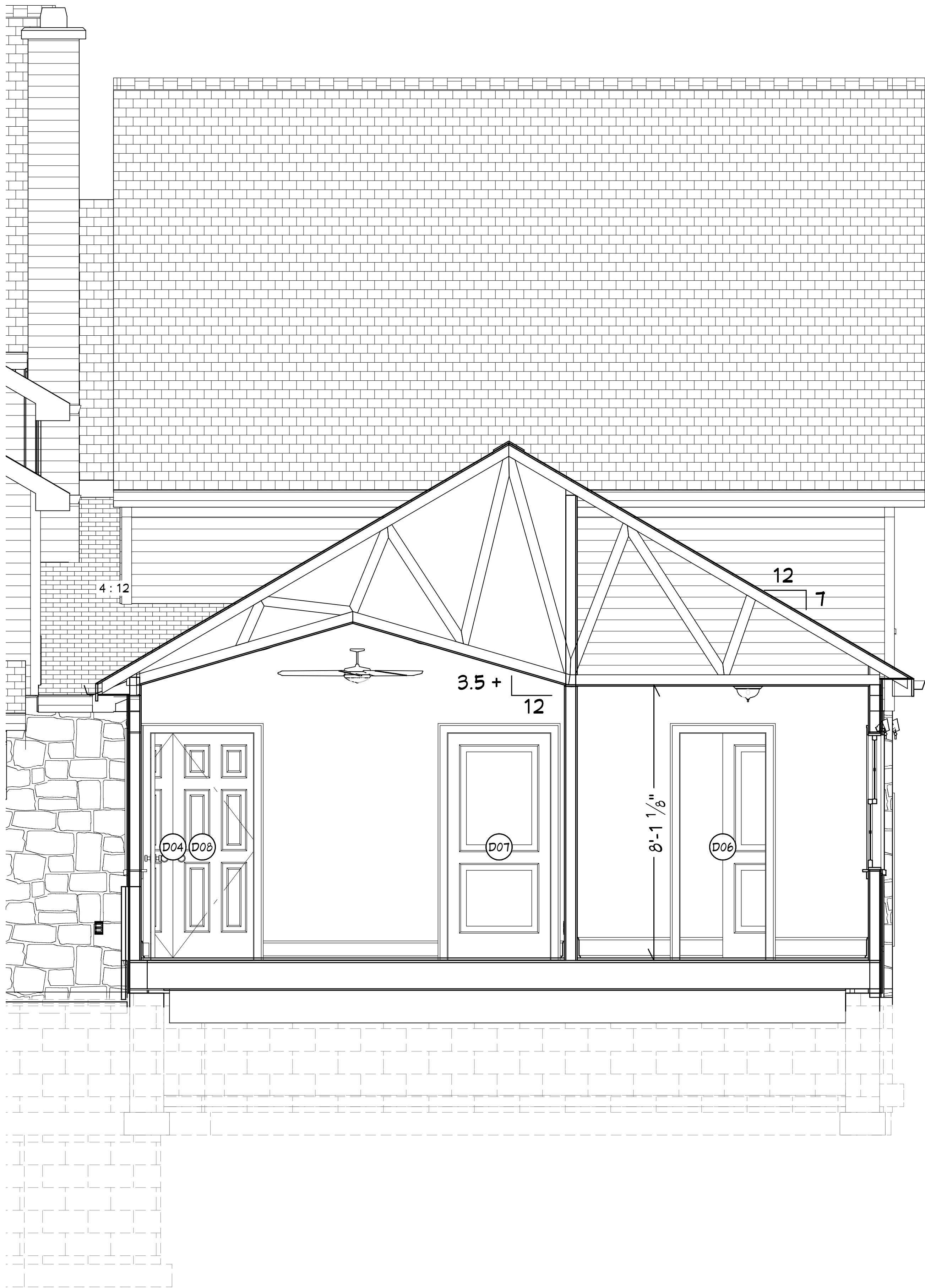
3 Section through Primary suite A-7 1/2 in = 1 ft
