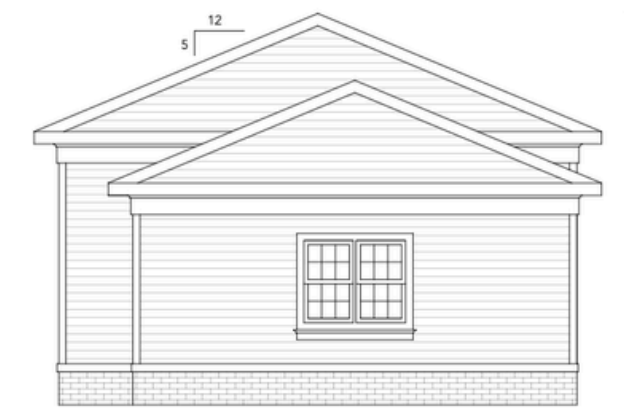
4 PROPOSED SOUTH (SIDE) ELEVATION 1/4" = 1'-0"
