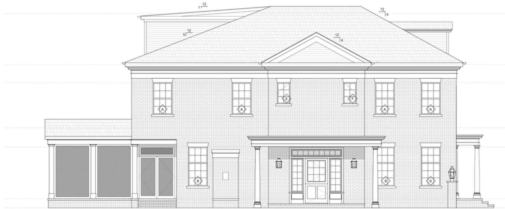
1 PROPOSED SOUTH ELEVATION 1/4" = 1'-0"
