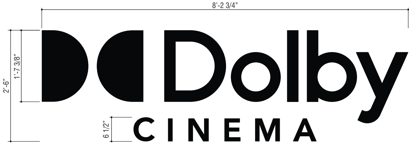
1 FACE LIT CHANNEL LETTER LAYOUT SCALE: 3/4"=1'-0" 20.6 sf
