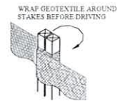
JOINING SECTIONS OF SILT FENCE DETAIL REFERENCE ONLY NOT TO SCALE
